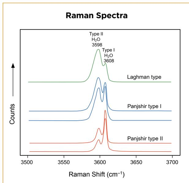
**Figure 9:** Raman spectra show variable band intensities corresponding to the different orientations of the water molecules in the channel structure (i.e. type I and type II H<sub>2</sub>O; after Huong *et al.* 2010) for emeralds from the three studied occurrences in Afghanistan. The spectra have been offset vertically for clarity.
