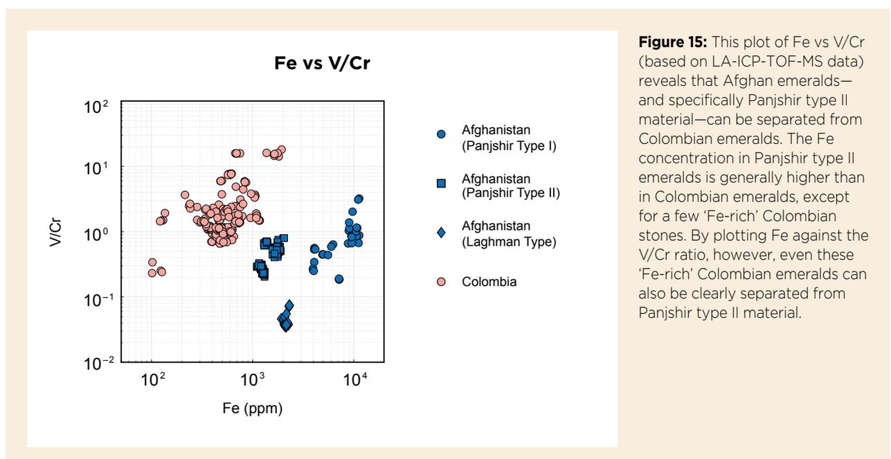
**Figure 15:** This plot of Fe vs V/Cr (based on LA-ICP-TOF-MS data) reveals that Afghan emeralds—and specifically Panjshir type II material—can be separated from Colombian emeralds. The Fe concentration in Panjshir type II emeralds is generally higher than in Colombian emeralds, except for a few 'Fe-rich' Colombian stones. By plotting Fe against the V/Cr ratio, however, even these 'Fe-rich' Colombian emeralds can also be clearly separated from Panjshir type II material.
