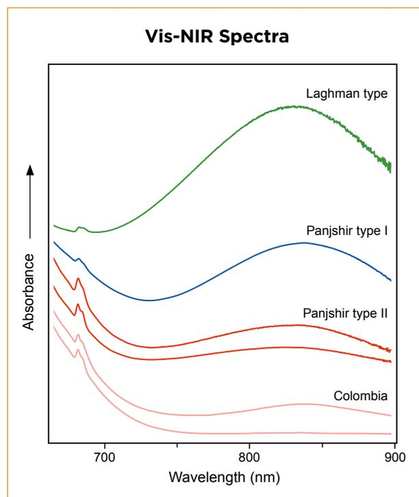
**Figure 13:** Polarised absorption spectra (o-ray) for the three Afghan emerald types in the red to near-infrared range show variations in the strength of the absorption band at about 830 nm, which is related to octahedrally coordinated  $Fe^{2+}$ . Panjshir type I and Panjshir type II emeralds show weak-to-moderate absorption, whereas stones from Colombia typically exhibit no such absorption feature. The spectra have been offset vertically for clarity.
