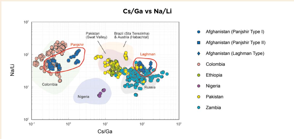
**Figure 19:** A plot of the ratios of Cs/Ga vs Na/Li, as proposed by Schwarz (2015) for showing genetic relationships between various types of emerald deposits, reveals that stones from Panjshir (specifically type II) and Laghman overlap with different emerald population fields. The coloured fields are from Schwarz (2015) and Giuliani *et al.* (2019).
