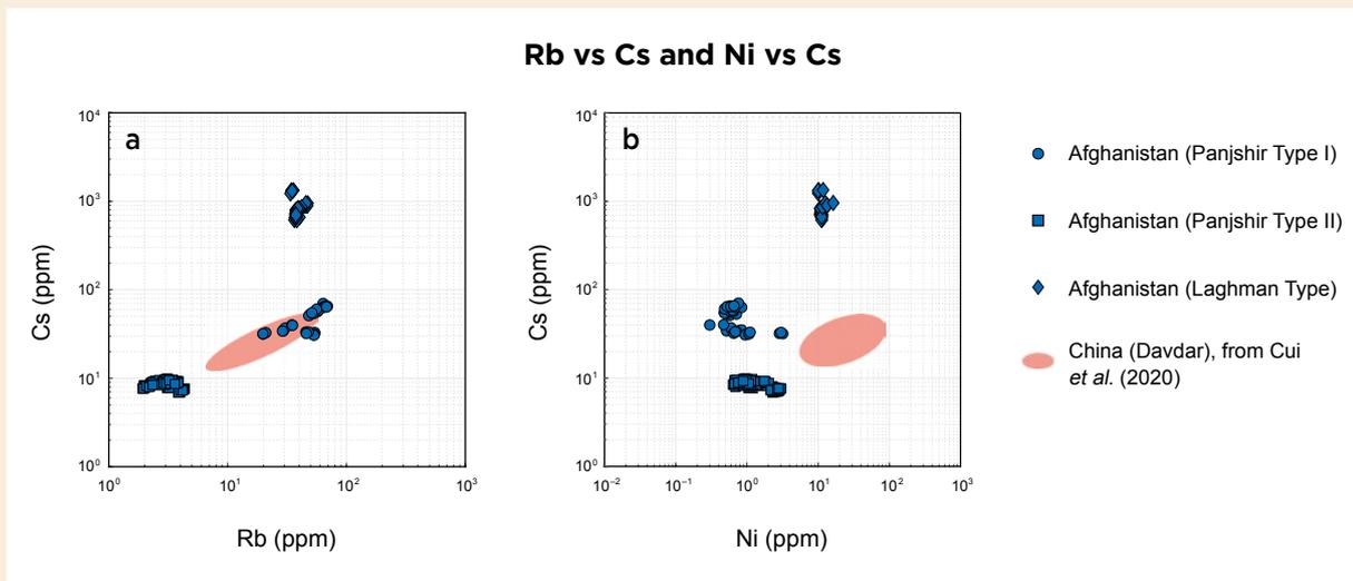
**Figure 18:** Trace-element data for Davdar emeralds (from Cui *et al.* 2020) are plotted together with analyses obtained in this study for the three types of Afghan emeralds. (a) A plot of Rb vs Cs shows a distinct positive correlation for both Davdar and Panjshir type I emeralds, with some overlap, whereas Panjshir type II and Laghman-type samples are clearly distinct. (b) A plot of Ni vs Cs clearly separates all three Afghanistan occurrences from Davdar emeralds.
