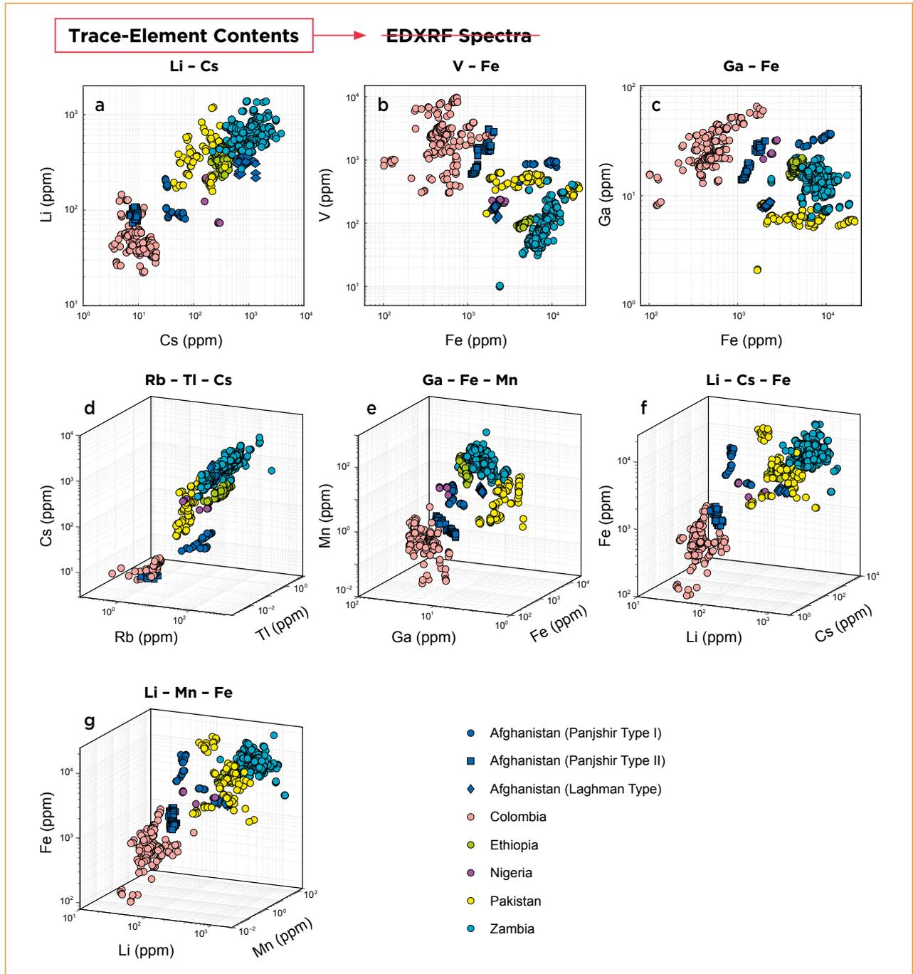
**Figure 17:** Scatter plots for various elements compare the three types of emeralds from Afghanistan with those from other important deposits, based on data collected at SSEF using LA-ICP-TOF-MS. Rotational video clips for each of the 3D scatter plots are available in *The Journal's* data depository.
