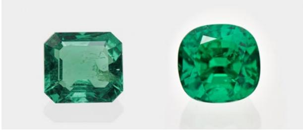
**Figure 14:** The appearance of an unusual Fe-rich emerald from Colombia (left, 5.77 ct) that shows a weak absorption band in the near-infrared region at about 830 nm is compared to a vibrant green Panjshir type II emerald (right, 4.50 ct). Composite photo by Luc Phan, © SSEF.
